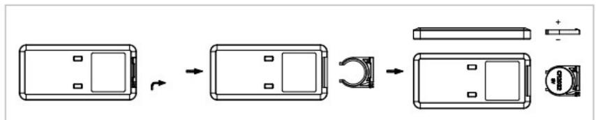
5. Replace the button cell with a battery of the same type (CR2025). Ensure correct polarity.
